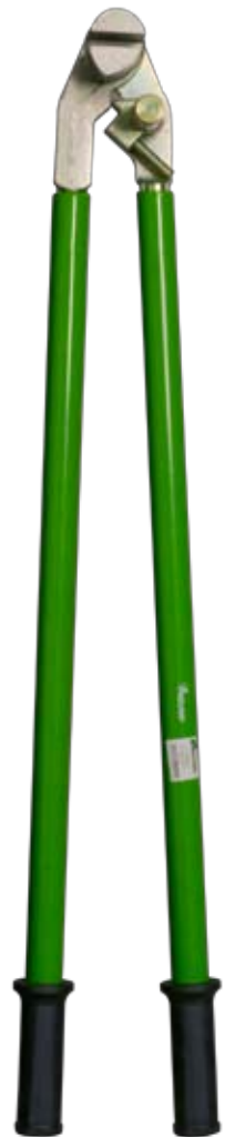
Bar Bender For bending Roof Bars as scene on page 1
