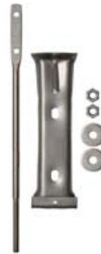
Hanger Unit, 5", 6" & 8", .060 Stainless Steel or Aluminum Brackets 3/16" x 11", 13", or 16" Stainless Steel Rods. 3/16" x 11" Aluminum Rods, Stainless Steel Nuts included (Optional Washers Available)
