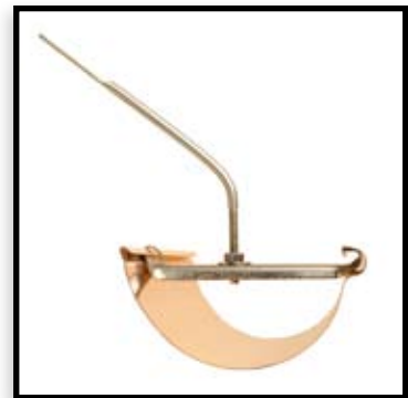
Hanger Unit, 5", 6" & 8", .060 Stainless Steel or Aluminum Brackets 3/16" x 11", 13", or 16" Stainless Steel Rods. 3/16" x 11" Aluminum Rods, Stainless Steel Nuts included (Optional Washers Available)
